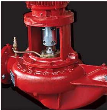
1) Split coupling with outside seal. Axially split coupling shown with coupling guard removed. Coupling bolts are still in place. Rotating element of seal is seen below the coupling, above gland plate.
