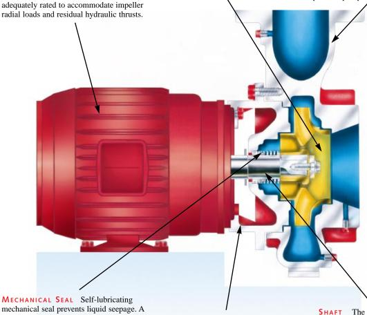
MECHANICAL SEAL Self-lubricating mechanical seal prevents liquid seepage. A carbon face rotating against a stationary 'O' ring seat provides positive sealing up to full design pressure. Higher temperature construction also available.
